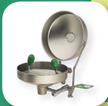
7460B Stainless Bowl Eyewash • Stainless Steel bowl • 2.5 gpm (1.25 ea) eyewash heads • Shown w/optional dust cover • Wall mounted
